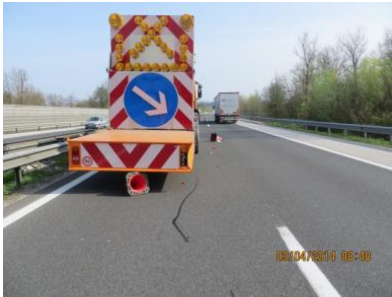
Figure 26: Damaged signal –on-trailer with crash cushion (3 April 2014)
