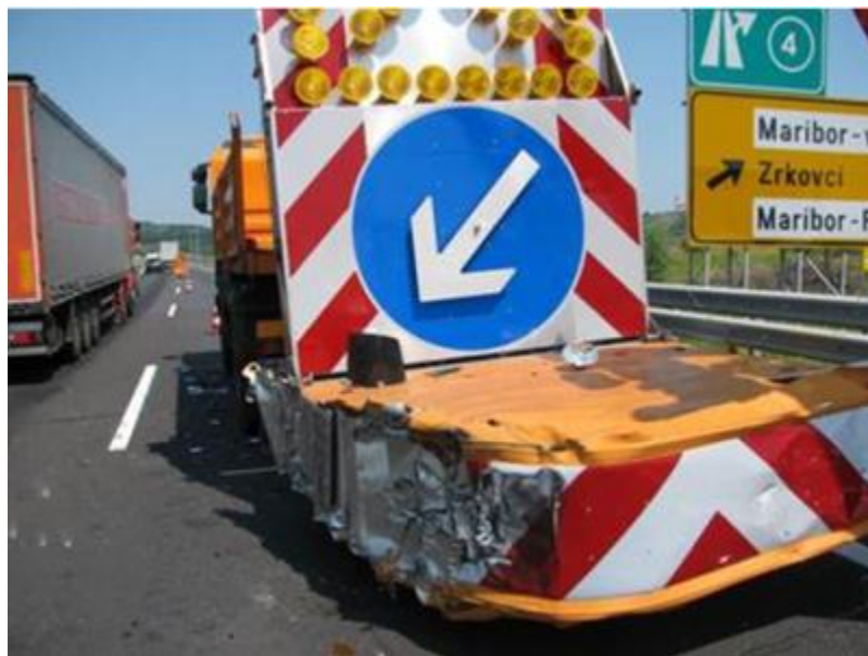
Figure 25: Damaged signal –on-trailer with crash cushion (18 July 2014)
